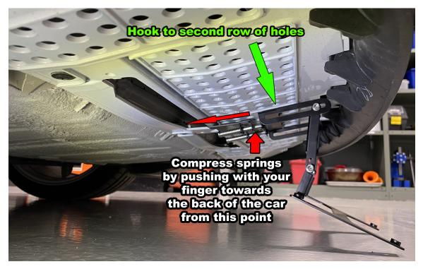
The first step is to fit the pre-assembled license plate mount to the car. The position of the plate holder is done in the next step.
