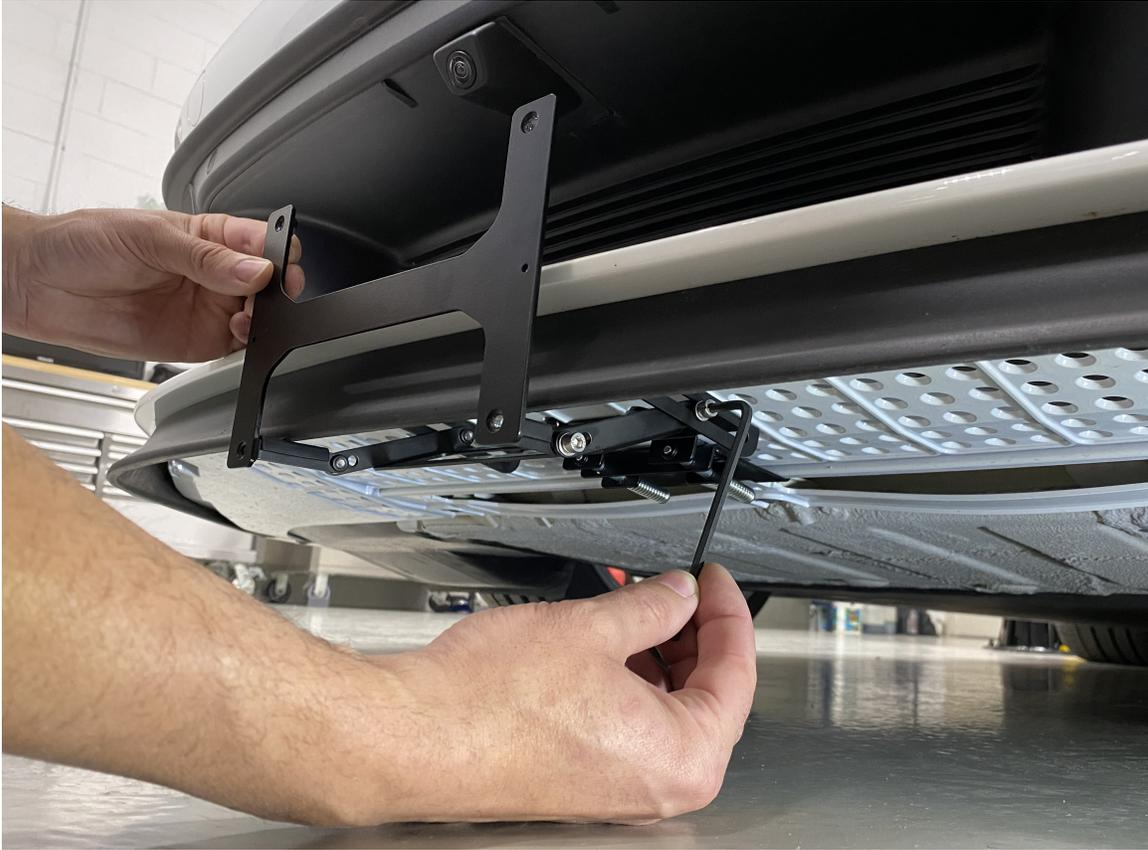
The plate mount is adjustable for both angle and distance. Using the included Allen head (hex) tool, loosen the 4 screws on either side of the plate holder and set the desired final position for the license plate holder. When the final position is achieved, tighten down the screws. It is easiest to first snug all the screws before returning to tighten them.
