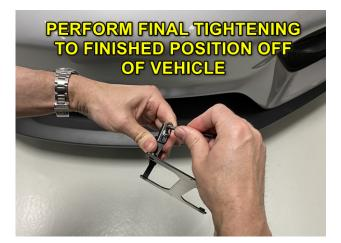
**Step 5d:** Re-install the mount by fitting the mount into the receiver (reverse of Step 5b) and by tightening the thumb nut firmly by hand.
