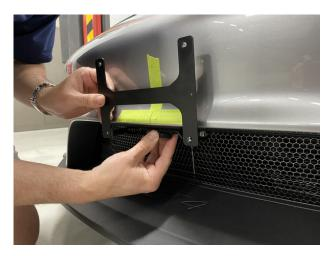
The goal is to find a position that is as deep as possible while still keeping the plate holder about 1cm (3/8") away from the surface of the bumper. Try to avoid locating the mounting base where two different surfaces meet. Be ABSOLUTELY SURE that there are no obstructions or raised surfaces that would keep the mount from mating 100% FLAT.
