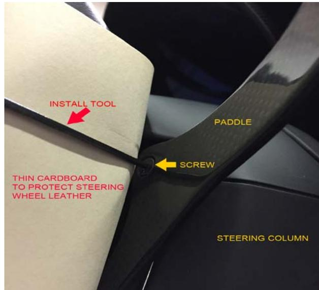
**CAUTION:** In rare instances the paddle screws are very tight from factory and require significant torque to loosen. If you find that the included install tool is twisting (when initially getting the fastener loose) more than a few degrees, you may wish to consider removing the steering wheel and using a shorter and stiffer Allen-head tool or you may risk breaking the included tool.
