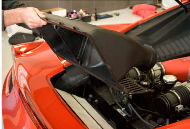
**Step 4:** Install the carbon airbox in the reverse order as the removal taking particular care not to drop the washers noted in Step 1.
