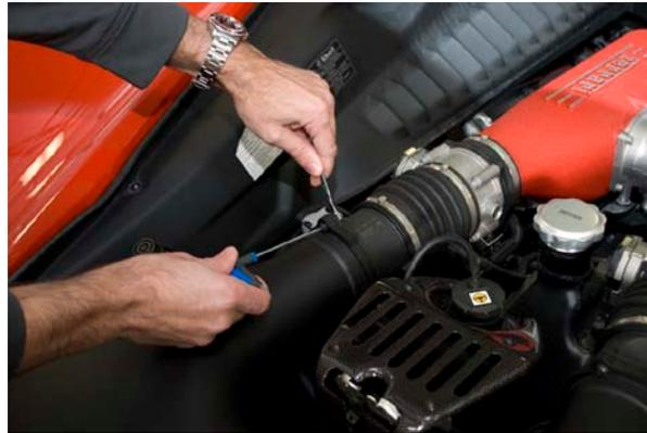
**Step 2:** Using a T20 Torx headed tool, removed the screws that hold the factory airbox in place around its perimeter.
