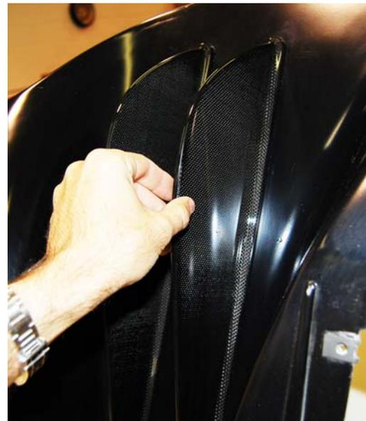
**Repeat Steps 2-8 for the other side of the diffuser. Double check the tightness of all mounting nuts and then re-mount the bumper in the reverse order as the removal.**
