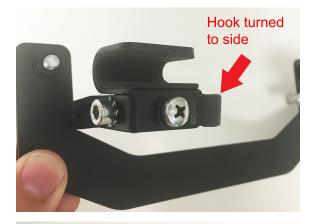
**Step 2:** Fix the mount in place by grabbing the serrated finger grips and pushing the rubber coated hook back on the spring loaded pin until the hook is clear of the backside of the grille. Once the hooks is clear, rotate the hook upwards until it is vertical and then gently release the spring pressure. Repeat this procedure for the opposite side.
