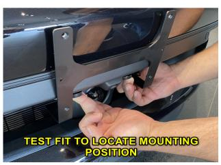
The goal is to find a position that is as deep as possible while still keeping the plate holder about 1cm (3/8") away from the surface of the bumper. Try to avoid locating the mounting base where two different surfaces meet. Be ABSOLUTELY SURE that there are no obstructions or raised surfaces that would keep the mount from mating 100% FLAT.
