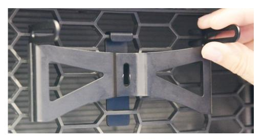
Step 3: Tightening the assembly to the grille
