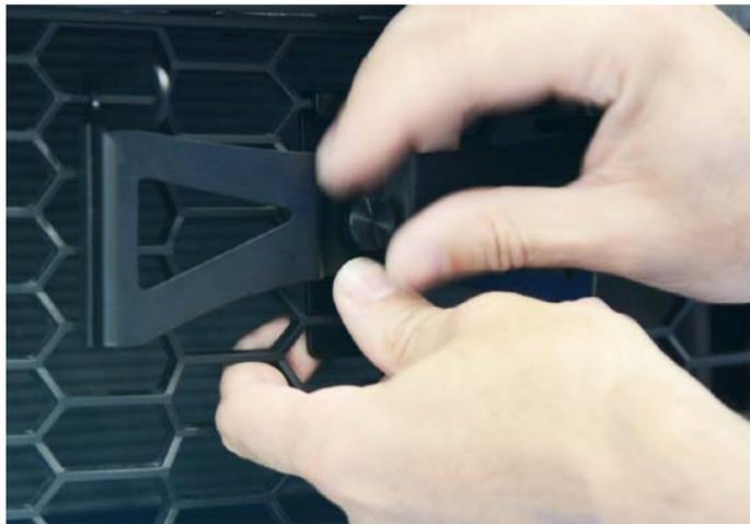
**Step 4:** With the mount securely attached to the grille use the included Allen head (hex) tool and loosen the two screws on either side of the mount. With these screws loose you can now set your preferred angle and distance for the license plate. Once the desired position is achieved firmly tighten down the two screws to complete the installation.
