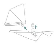
**5.** Adjust the footrest on the seat unit so it is at a right angle to the seat frame.
