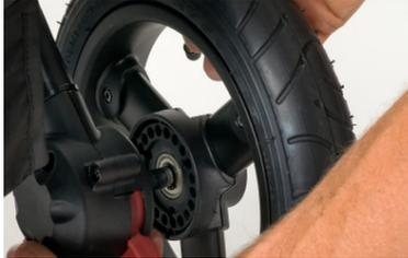
To **remove** a wheel, press the button on the wheel hub cap and pull outwards.
