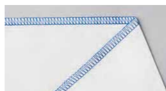
3-Thread Overlock This basic stitch of overlock prevents fabric from fraying.
