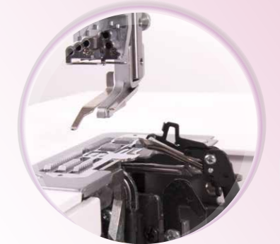
Sturdy looper channels with folding auxiliary looper
