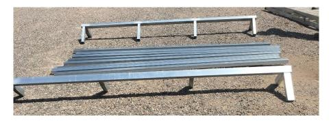
2. Join 4 x cross members to main frame, ensuring the joiners on each corner are all facing the ground
