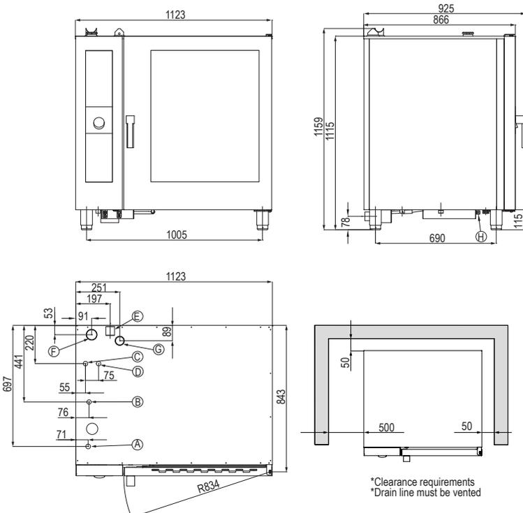
**Heat Source:** 500mm clearance from an external heat source is required in order to protect the oven control components and allow access to the service panel. For clearances under 500mm, it is mandatory for Stoddart heat shields to be fitted while still maintaining a minimum clearance of 300mm to provide access to the service compartment. Failure to adhere to minimum clearances may void the oven warranty or add service costs due to lack of access.
