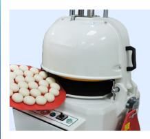
Simply insert your rounding plate with dough into the machine and the machine will automatically press the dough out to the edge of the plate, cut and divide the dough into equal portions, then round. The machine allows you to create different types of rolls with varying weight ranges and sizes.
