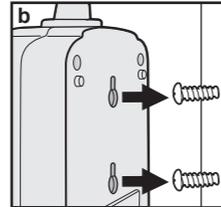
b. For a more secure mounting, use the two MOUNTING HOLES on the back of the timer.
