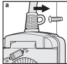
a. Using a screw or hook (not included), secure the MOUNTING TAB at the top of the timer to a wall or post.
