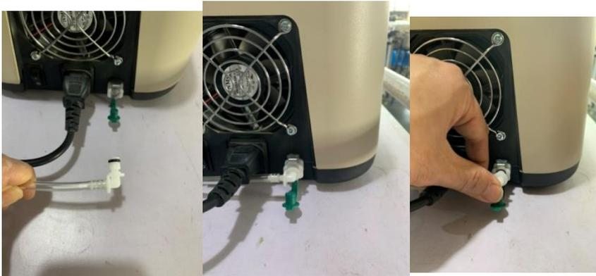
3. Check all connections and confirm they are secure. Then open the switch of the transfill and start filling with oxygen.
