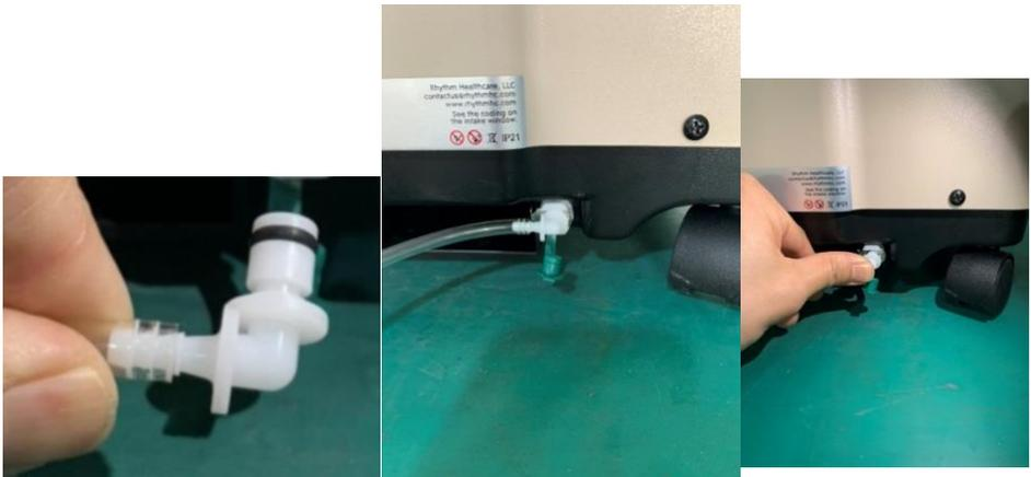
Press the metal shrapnel on the port of the transfill. The plastic plug will loosen and pop out.
