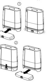
Important: The first time you charge the battery, be sure to charge it fully. Do not use the DC power cord for initial charge; instead use AC power.
