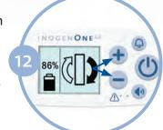
Press and hold the plus (+) and (-) minus buttons for 5 seconds. The screen will display "sieve reset" message. Release buttons once message is displayed on screen.
