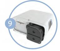
Insert column assembly into the Inogen One® G5 concentrator.
