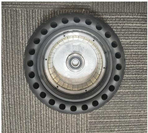
Carefully lever the tyre onto the rotor, being careful not to damage or scratch the motor. It can help apply pressure to the tyre while levering with either your hands or your foot, which can be quite tricky solo. So it could be helpful to have a partner for this step.
