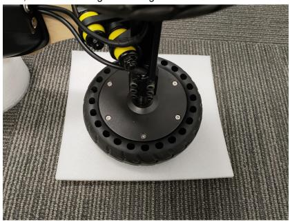
Use an appropriately sized phillips head screwdriver and remove the 6 hub cap bolts on the side of the wheel. An appropriate sized screwdriver, will fit into the screw/bolt leaving very little gaps around the screw head, see picture below:
