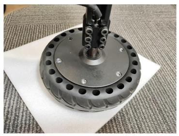
Flip the board over 180 degrees, so the the wheel you are changing is off the ground
