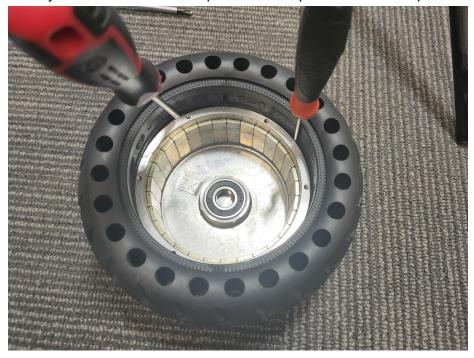
Once you have levered a small section of the tyre around the entire motor, you can push the tyre onto the rotor. Or use a rubber mallet to tap the tyre over the rotor, using a circular motion around the edges.
