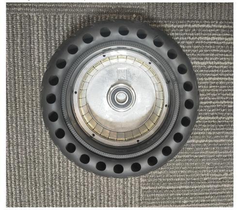
Line up the new tyre with the rotor (be sure to have the tread face the correct direction).
