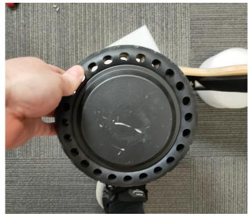
**NOTE:** The motor wheel is significantly harder to remove than the front wheels. This is due to the rotor being held to the stator with strong magnets, so you may require a partner to assist with this step.
