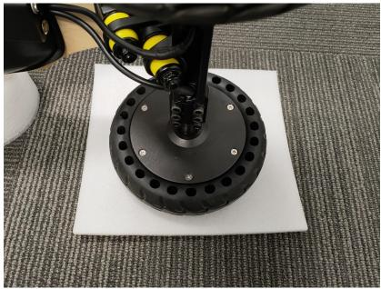
Use an appropriately sized phillips head screwdriver and remove the 6 hub cap bolts on the side of the wheel. An appropriate sized screwdriver, will fill the vast majority of the screw, see picture below:
