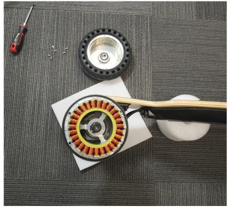
The tyre is a very tight fit, so may take some patience and effort to remove. Using the tyre levers or flat head screwdriver, carefully lever the tyre off the rotor little by little around the edges until the entire tyre is removed or is loose enough to remove by hand.
