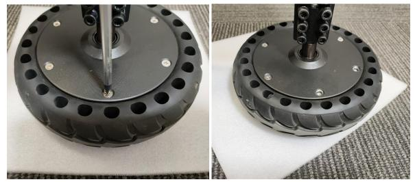
Once all 6 bolts have been removed you should now be able to remove the outer rotor of the wheel.
