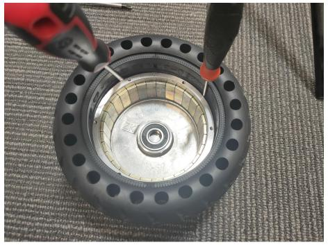
Once you have levered the tyre a small section of the tyre around the entire motor. You can push the tyre onto the rotor. Or use a rubber mallet to tap the tyre over the rotor, using a circular motion around the edges.
