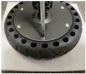
Once all bolts are finger tight. Tension each bolt evenly in a circular pattern or in a star pattern (star pattern recommended). A reference to the tension patterns is available towards the end of this document.
