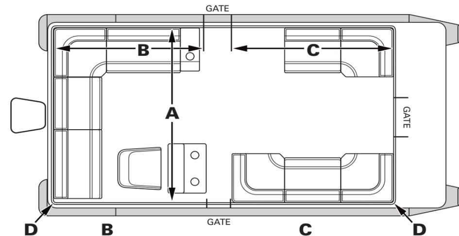
Measure "A" distance between the Port and Starboard rails. (Allow for 1" extra spacing for vinyl and foam). Most boats measure 89" to 93" wide.
