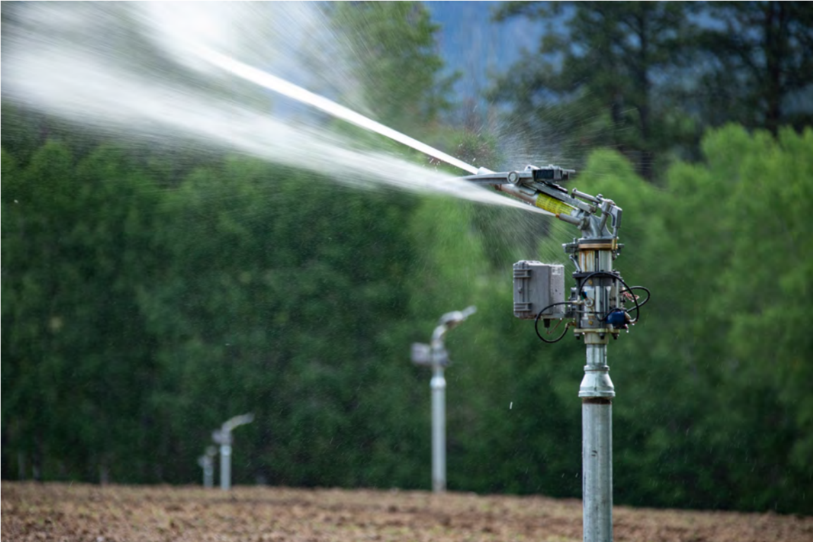
Figure 8. TWIG® Wireless Automation with Nelson control valves helps achieve precision irrigation with Big Gun® sprinklers.
