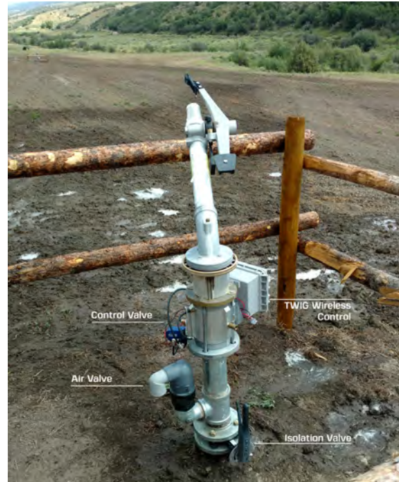
Figure 18. F150 Big Gun® sprinkler with Nelson 800 Series Control Valve and TWIG® Wireless Controls, installed on a riser with butterfly valve for isolation, and Nelson ACV200 continuous acting air relief valve.
