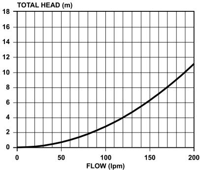
Note: Head loss through controller is for horizontal (90°) outlet and with integral check valve in place.
