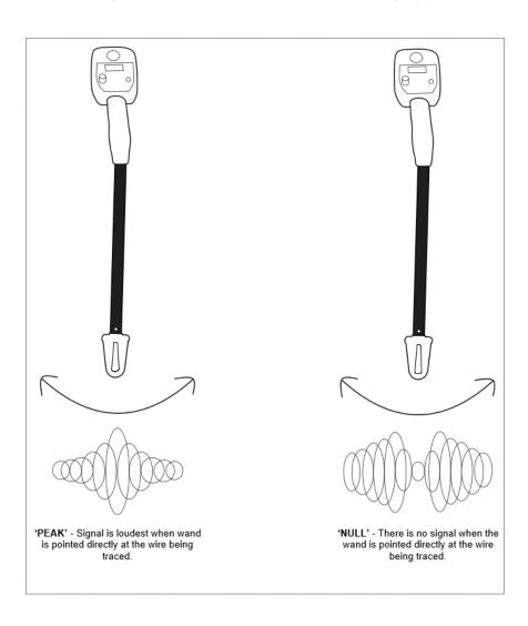
Tracing Live Electrical Lines using Passive Mode - The Pro871C<sup>™</sup> receiver has the capability of detecting live electrical AC lines in the ground without connecting to them. This is known as passive mode. In passive mode, no transmitter is used. DO NOT ATTEMPT TO CONNECT THE ALLIGATOR LEADS OR ANY OTHER PRO871C<sup>™</sup> COMPONENT TO LIVE ELECTRICAL LINES. DEATH OR INJURY COULD OCCUR.
