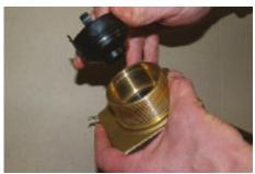
2. Low Pressure Valve (LP) - Remove the High Pressure insert to make the valve Low Pressure.
