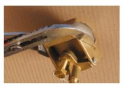
5. Tighten Valve - Tighten the body of the valve using a pair of multigrips or a spanner. Ensure the body is in an upright position so that the lever arm moves in a vertical position.
