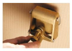
6. Adjust the float level - Adjust the floatlevel by screwing the adjusting bolt in or out of the cam. Screwing the bolt out lifts the water level, screwing it in lowers the water level. Once the correct level is found ensure the nut is tightened to stop the adjusting bolt from moving. Please note if valve is weeping then screwing adjusting bolt in an additional half turn should ensure shut off is achieved.
