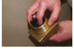
7. Removing the HP insert onceinstalled - Use a screw driver to remove the insert lugs from the valve body. Ensure all four lugs are loose from their position. Then pull the insert from the valve body. The valve is now suitable for Low Pressure applications.
