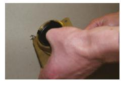
3. High Pressure Valve (HP) - Push insert into the valve body until lugs click into place. Valve is now suitable for High Pressure applications.
