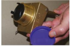
Remove Protective Cap - Remove protective cap and dispose. Note the high pressure (HP) insert in the valve body.
