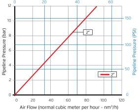
Air relief and intake charts are based on actual measurements, made in Bermad Air Flow test bench, according to EN-1074/4 standard and refer to Side outlet.
