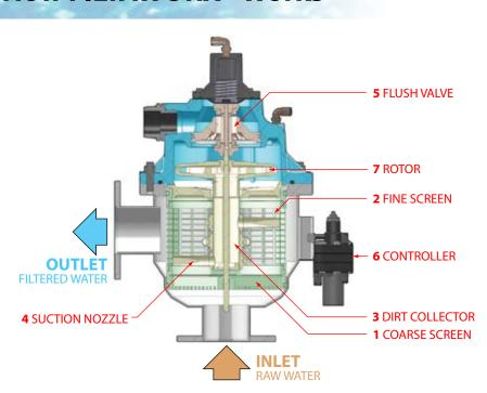
During normal filtering mode the raw water enters the Inlet of the filter, passes through the Coarse Screen (1), (this removes large debris that may obstruct the lower mechanism). Water then travels to the inside and through the Fine Screen (2) to the Outlet.
