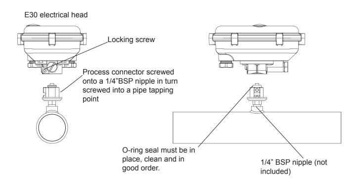
Typical tapping point on a section of pipe
