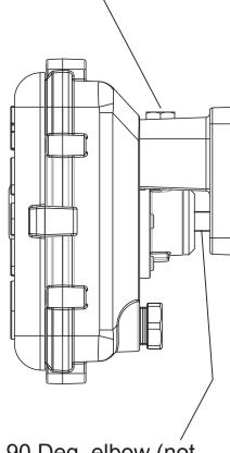
Screw a 1/4"BSP 90 Deg. elbow (not supplied) into the process port on the E30. The inlet port on the elbow must be aligned downward to accept a capillary tube adaptor and to stand clear of the wall.
