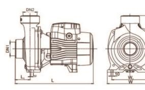
DN1 DN2 L (mm) W (mm) H (mm) L1 (mm) L2 (mm) W1 (mm) 2' 2" 371 263 3.5 206 59 166
