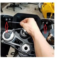
8. Using the 4 nuts that secured the mirrors, thread the nuts onto the mirror block offs to secure them in place. Tighten them with a 10mm wrench or socket wrench.
