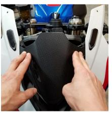
9. Reinstall cover make sure the bottom cover hook is in place and push gently but firmly over the 2 push clips until it pops into place.
