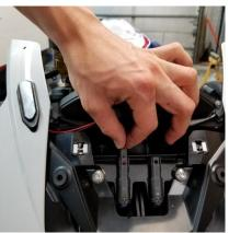
5. Using a 10mm wrench or socket wrench, remove the 4 nuts (2 per mirror) from the underside of the upper fairing. Set the 4 nuts aside as they will be reused. Remove Mirrors
