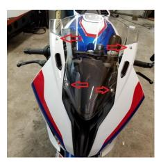
10. Reinstall windscreen with the T20 Torx driver. The bolts with the plastic washers go on the upper locations to protect the paint work.
