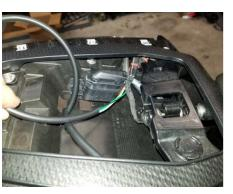
18. The 2 connector leg of the wire harness threads underneath the 2 wires and out the clutch side of the trunk. Connect to the OEM harness female plug.
