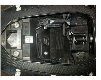
19. Tuck/ route the wire harness wires using the routing tabs like the OEM harness.
