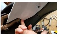
3. On the underside of the tail fairing, wedge your finger under the fairing by the sub frame.
