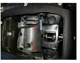
10. Thread the wires out and free as much as you can. they all run through the trunk into a single hole at the rear
