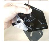
\*\*\* MUST APPLY MEDIUM STRENGTH THREAD LOCKER (Blue Loctite) to the little M4 fastener.
