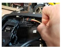
17. The single connector leg of the wire harness threads under the throttle side of the trunk. Connect to the OEM harness female plug.
