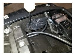
15. Remove only the rearward T20 Torx screw. Be super careful to not drop it into the abyss of the tail. You may want to shove a rag under the seat latch to catch a dropped bolt.
