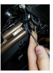
8. Disconnect 3 wire connectors. 2 on the clutch side of the bike and 1 on the throttle side of the bike. They are behind the plastic grill/mesh under the tail.
