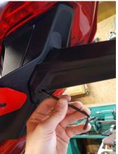
1. Remove the 2 fasteners retaining the plate arm
