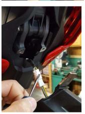
3. Use a little flat head screwdriver to disconnect the plate arm wire connector
