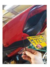
9. Retighten the tail fairing fasteners
