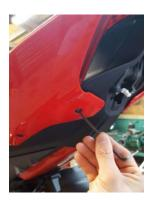
5. Loosen, don't remove the4 bolts that hold tail fairing inplace to allow for wiggleroom and alignment
