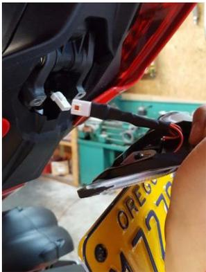
7. Connect tail tidy wire connector to motorcycle wire harness. Gently tuck the wires into the tail make sure there is nothing being pinched
