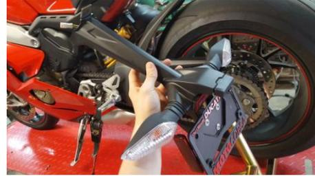
5. Loosen, don't remove the 4 bolts that hold tail fairing in place to allow for wiggle room and alignment
