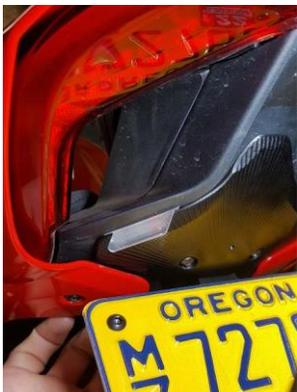
With the tail fairing bolts loose, you can wiggle / move the fairing if need to help place the Tail tidy.
