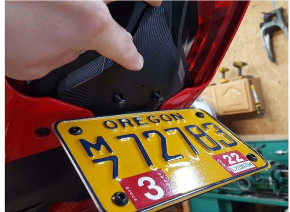
8. Hand thread the supplied Tail Tidy mount bolts M5x16mm once threaded tighten with
