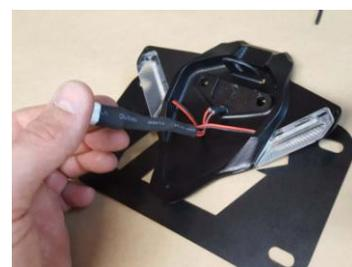
Apply Medium strength thread locker (Blue Loctite) to the little M4 fastener.
