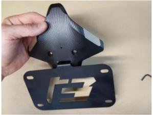
Apply Medium strength thread locker (Blue Loctite) to the little M4 fastener. Center the plate bracket and tighten bolt snugly using 2.5mm Hex wrench
