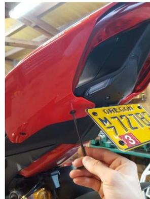
9. Retighten the tail fairing fasteners
