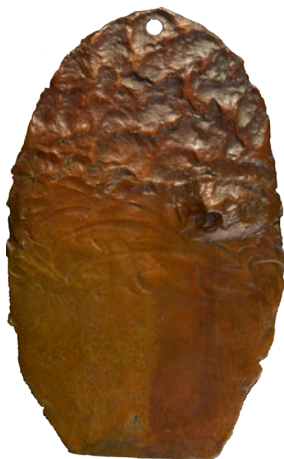
Above: Traditional Liver of Sulfur and Ferric Nitrate patinas on bronze
