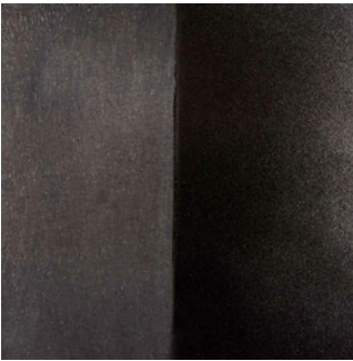
Above: Black Magic on the left. Black Magic and 2 coats of Black Patina Stain on the right.
