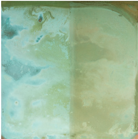
Traditional Tiffany Green on copper Clear Guard Matte (left) Age-It with Clear Guard Matte (Right)
