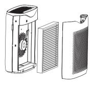
Take out the old filter by pulling the tab. Unwrap a new one.
