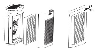
2. Reinstall the HEPA filter. Make sure the pull-tab is facing outward. Then reinstall the front shell.
