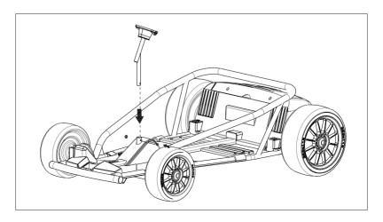
②.Insert the steering axle from the bottom to the car body and steering wheel strut, until the top of the steering axle extends out the steering wheel strut.
