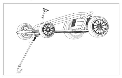
6. Steering wheel assembly Insert the steering wheel to the steering axle, fix them with M5\*50 screw and M5 locknut.
