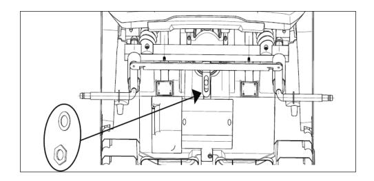
For each side of the vehicle, from inside out, slide M12 washer, front wheel, then M10 washer. Secure the connection with M8 nut, then place the nut cap.
