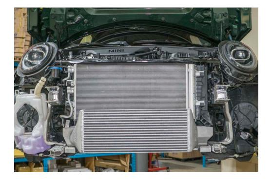
With the provided hardware install the washer and 5mm allen to secure the intercooler on the bottom mounts.
