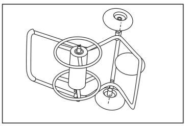
**D.** Place the unit on its side to assemble the hose reel to the frame.
