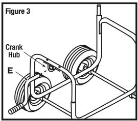
**4.** (SEE FIGURE 4) Place hose reel (D) into frame assembly (A). Insert end of crank stem from hose reel (D) onto crank handle (E).
