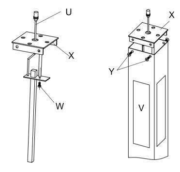
As shown above, fasten the lamp (U) to the cover (X) with a small screw (W). The lamp wire passes through the center hole of the cover (X); and the cover and the post are fixed together with the tapping screw (Y).
