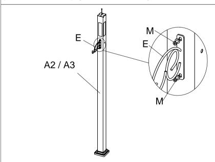
2. Screw the hook (E) to the post (A2), (A3) by screw (M).
