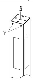
Remove the solar panels, covers and beams; then Screw out the four screws (Y) on the post with a cross screwdriver.
