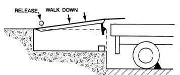
3 To return the leveler to stored position, pull the back release ring. Release the ring as soon as the lip is fully retracted.
