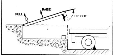
2 With the lip fully extended, **pull** the **front** release ring to retract the safety legs as the leveler is walked down.
