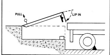
With the lip fully retracted and clear of the truck, walk down the leveler to the stored position.
