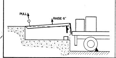
With the leveler above dock, pull the front release ring to retract the safety legs as the leveler is walked down.
