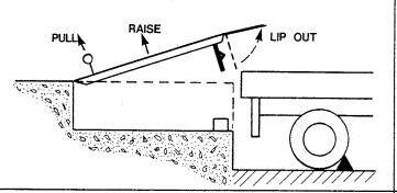
When the lip is fully extended release the ring. Walk down the leveler to the truck bed.
