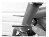
2. Loop the U-bolt around your head tube. There are three sizes. Use the smallest that fits.
