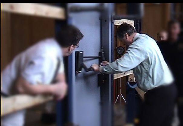
Inside view after 20 mins and the mechanism has jammed preventing entry.
