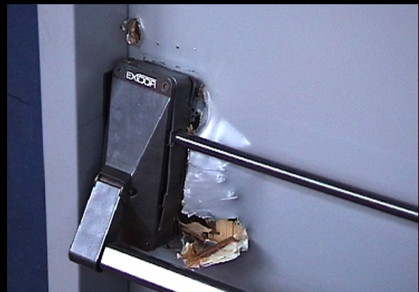
Inside view after 15 mins and the 4th bolt is still holding the door secure.
