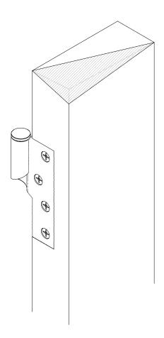
Example: Rise 10mm – Gap 3mm + 1mm tolerance = Plane allowance 8mm
