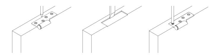
The leaf with the pin must be fitted to the frame, with the pin pointing upwards. At the determined spacing, position the non pin hinge leaf to the door so that the edge of leaf by knuckle is flush with edge of door and mark around leaf. Repeat at each hinge position. Mortice out door to equal the thickness of the hinge leaf. The mortice should be smooth and any shavings or swarf must be removed.
