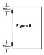
**Figure 5** - The standard practice for fitting rising butt hinges. Assistance should be sought from manufacturer in circumstances where a 3rd hinge is required as a co-axial point must be maintained.
