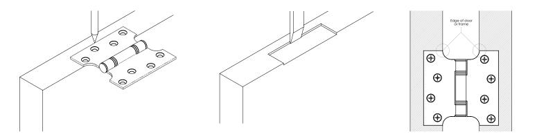
Always refer to manufactures installation instructions for any special requirements. If intumescent pads are being fitted behind the hinge leaf, ensure to increase the mortice depth accordingly.
